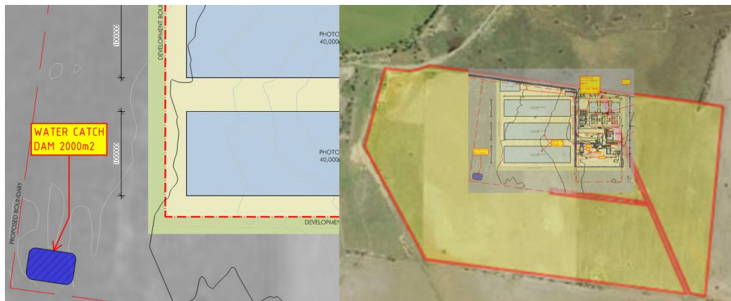
Figure 7 - Proposed Catch Dam South-West of PV Installation
